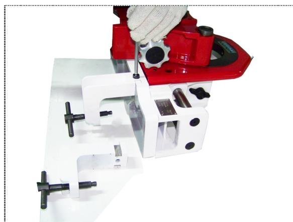
**Step 2:** Align square top of motor with the trough inside gear hosing then put it into the gear hosing and get fastened onto the work bench
