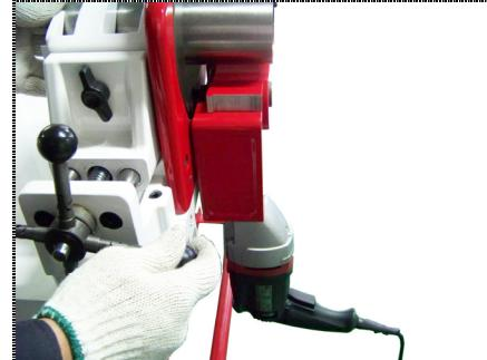
**Step 3:** Apply lubricant to the saw blade for each cut.
