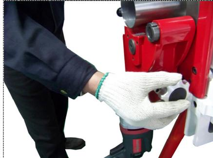
**Step 2:** Insert the tube, to the position where the blade would cut off the tube, and then fasten the clamp.
