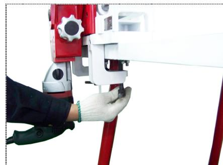
**Step 3:** Install the saw blade depending on application.
