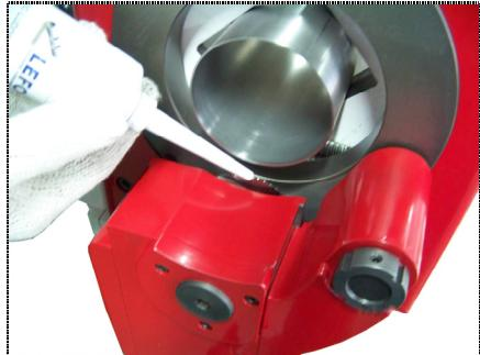
**Step 4:** Rotate the motor clockwise about 45° until the saw blade reaches the tube. Rotate the hand wheel to adjust the cutting depth, normally there is about 1-2mm teeth length into the tube. Then keep rotating the motor to finish the cutting.
